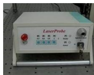
Fig. 7. The LASERPROBE system for blood sampling.
