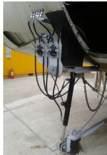
Fig. 13. Electro-hydraulic side tilt subassembly
