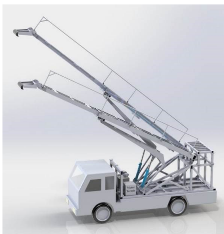
Fig. 7. Hydraulically actuated assault ramp - a 3D sketch
