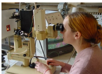
Fig. 2. MicroLASER x-y with Nd:YAG laser
