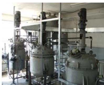
Fig 4. Pilot plant installation used for biodiesel production from rapeseed oil
