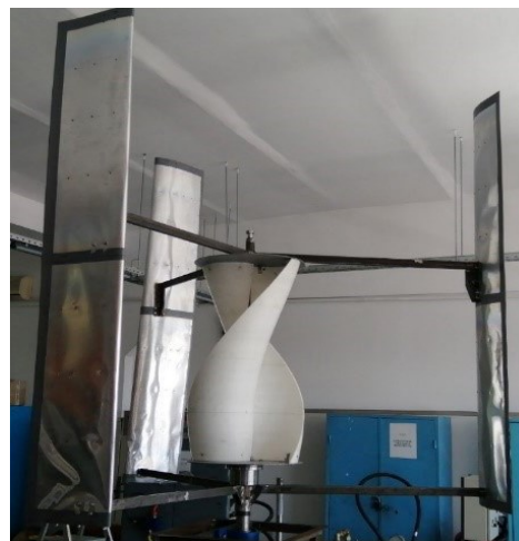
Fig. 2. Combined turbine with start at low wind speed
