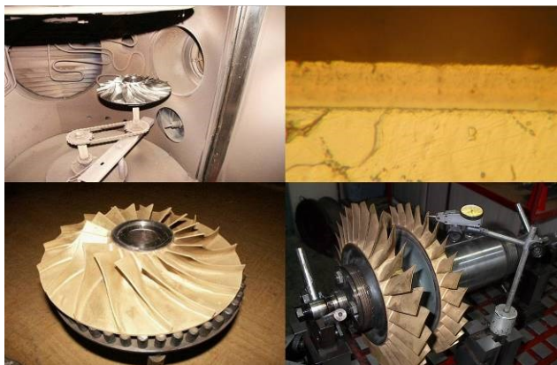
Figure 4: Images of the rotor blades after deposition, before and after being mounted on the bench test of the centrifugal air compressor. The image in the right up corner is presenting a transversal section of the multilayered coating.
