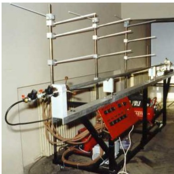
Figure 1: The LDS system with mass spectrometer, vacuum system, system for gas mixing and computer
