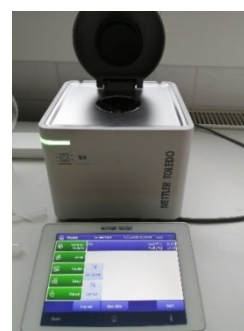
Fig. 14. Refractometer Mettler Toledo used for analysis of ethanol
