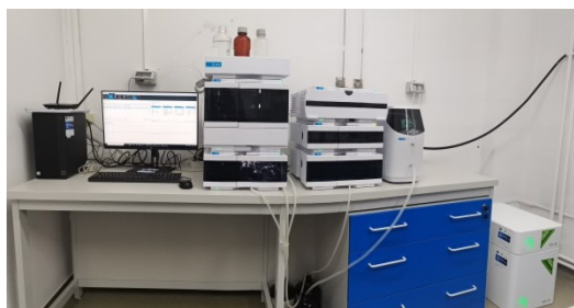
Fig. 21. UHPLC with DAD, RI and ELSD detectors used for sugar analysis
