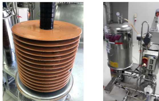
Fig. 8. Filtering layers and the filtration compartment
