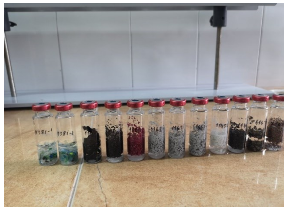
Fig. 16: Intermediary treatment of e-waste samples for identifying the plastic compounds using gas-chromatography and mass spectrometry
