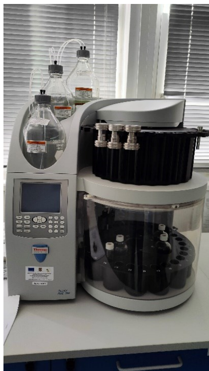
Fig. 4 Dionex AS 350 Accelerated Solvent Extractor
