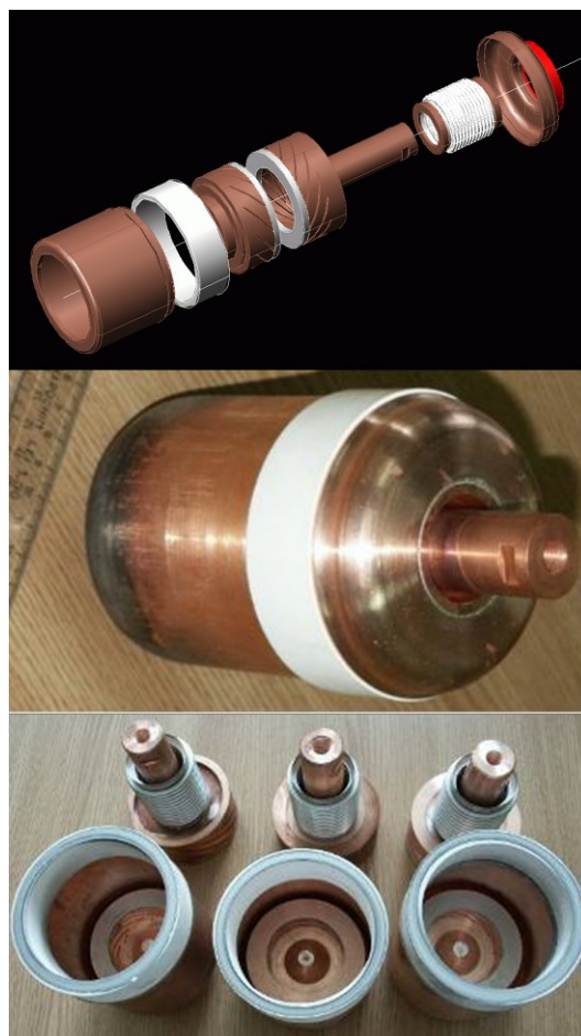
Figure 3: Images of the QC: from the design, to the fabrication, parts before assembling and the prototype
