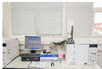
Fig. 13. GC-FID used for analysis of superior alcohols
