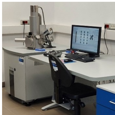
Fig. 3. SEM TESCAN VEGA 3 SBU microscope with a Quantax EDS XFlash detector
