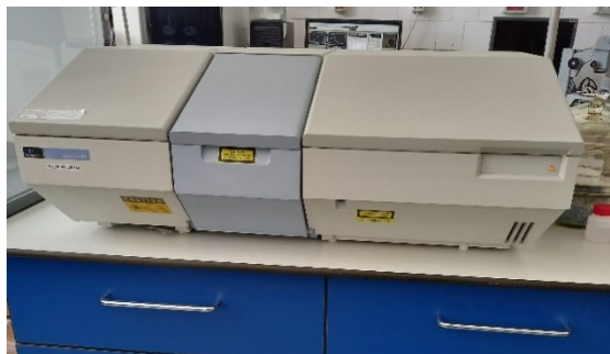
Fig. 4. Perkin Elmer Spectrum BX II Fourier transform infrared spectrometer.
