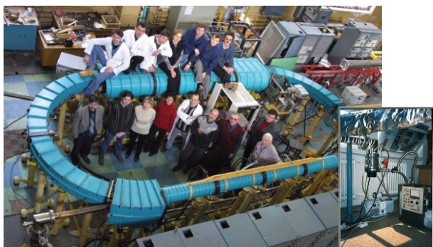
Figure 2: The UHV system for forming and transport of positrons and electrons in LEPTA, installed at JINR Dubna.
