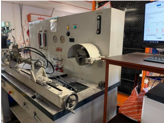
Fig. 23. Hydraulic steering boxes test bench
