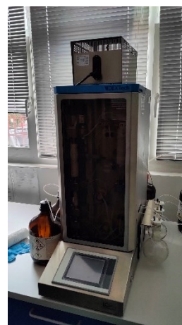
Fig. 5 Sample clean-up system (DEXTech 16)
