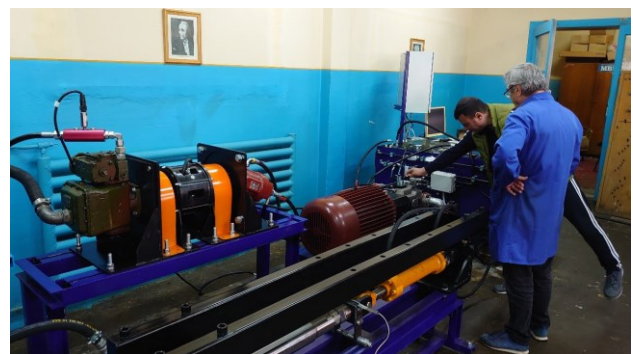
Fig. 8. Bench for hydrostatic drives
