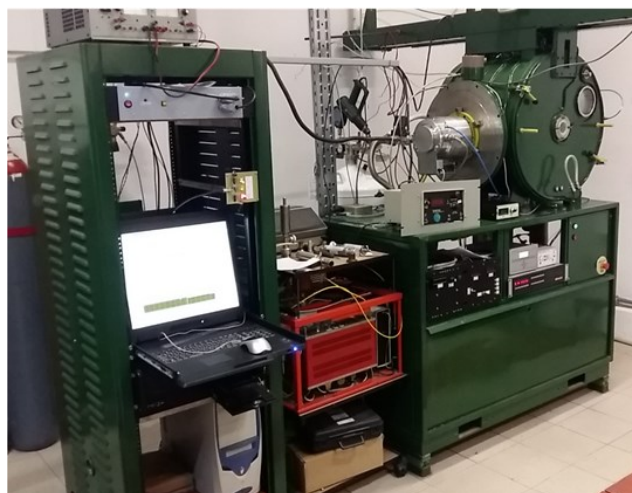
Figure 23. Facility for high vacuum testing and thermal cycling (TVAC)
