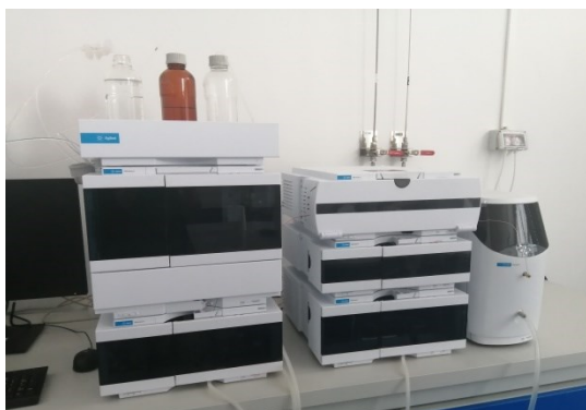
Fig. 14. UHPLC liquid chromatograph used for carbohydrates and bio-products analysis obtained from lignocellulosic biomass (Agilent 1290 Infinity II Prime LC)
