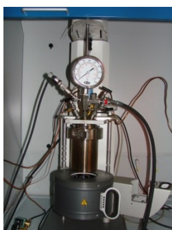
Fig. 10. Parr reactor used for the pretreatment process
