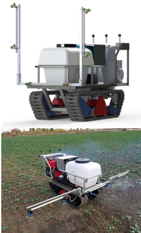
Fig. 18. Self-contained spraying platform - a 3D sketch and actual equipment
