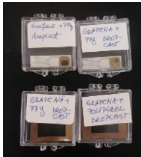
Fig. 19. Different types of gas sensors developed for the analysis of CO 2 from atmosphere (graphene and polypyrrole).
