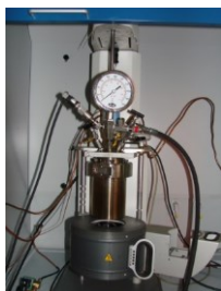
Fig. 9. Parr reactor used for the pretreatment of vineyard wastes
