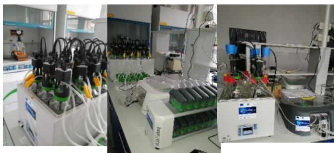
Fig. 7. The Automatic methane potential Test System (AMPTS II) (Bioprocess Control) used for biogas production and analysis
