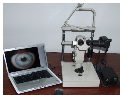
Fig. 3. The FOTOBIOFTAL biomicroscope with image acquisition, processing and storage, used in eye surgery or iridology.
