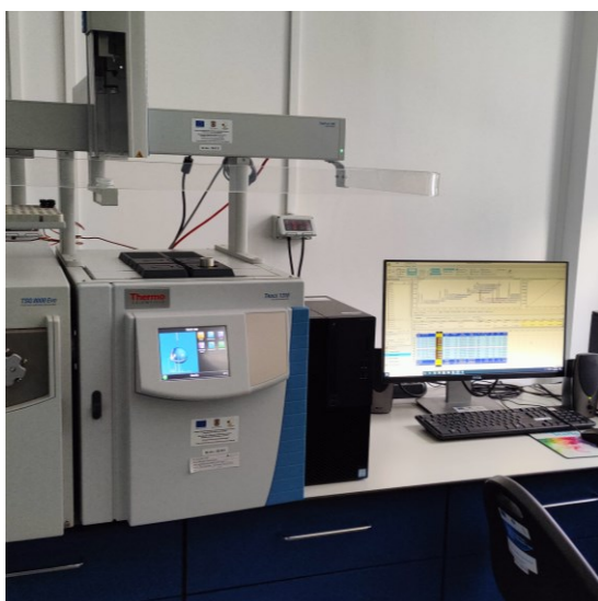
Fig. 3 GC Tracer 1300 series +TSQ 9000 ThermoFisher
