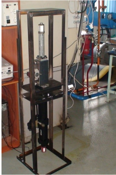
Fig. 20. Test bench for servo cylinders as part of an active heave compensator
