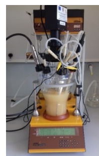
Fig. 9. Bioreactor Lambda 25 used for fermentation processes
